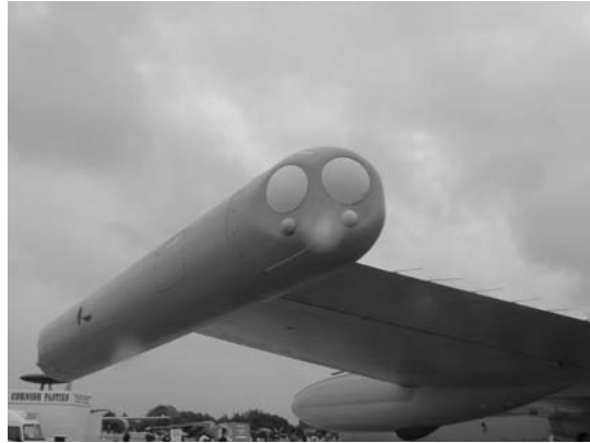
Figure 6.12 Wing-tip ESM pod installation – Nimrod MR2.
