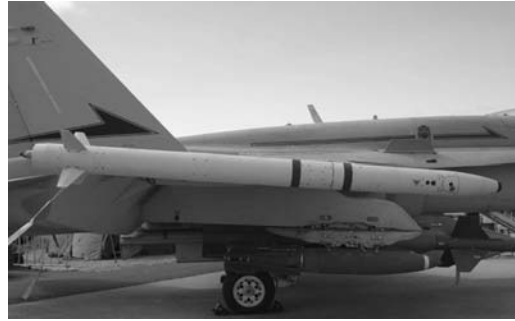
Figure 9.22 AIM-132 ASRAAM. (BAE SYSTEMS © 2005)
