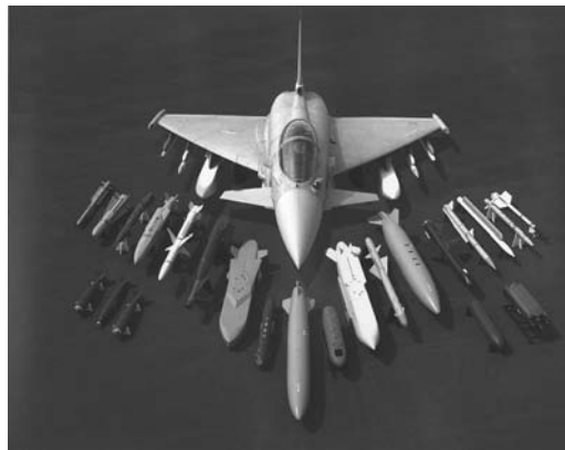
Figure 9.12 Typhoon weapon carriage options. (BAE SYSTEMS)
