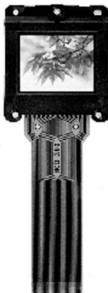
Figure 11.55 Typical transmissive LCD device.
