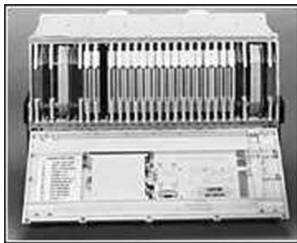
Figure 9.3 MLU modular mission computer.
