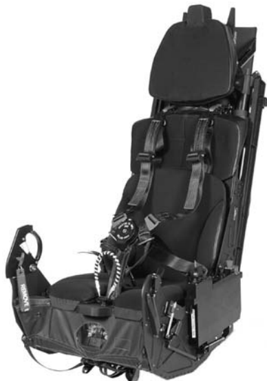
Figure 10.13 Modern military ejection set – F-35 JSF Seat. (Martin Baker)
