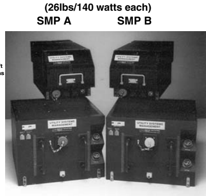
(26lbs/140 watts each) SMP A SMP B SMP C SMP D (44lbs/230 watts each) System Total: 140lbs 740 watts
