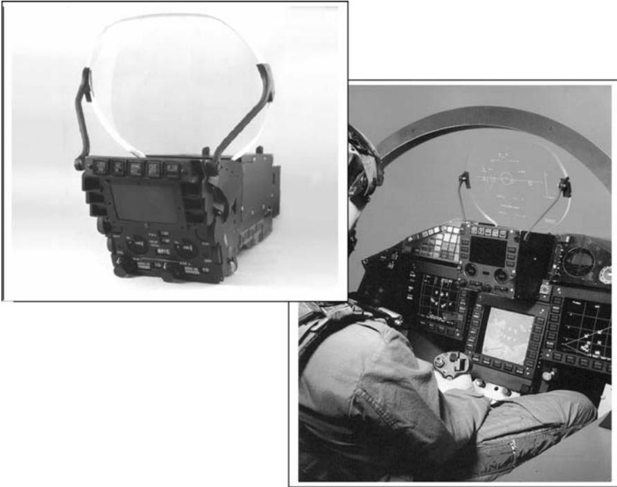
Figure 11.19 Eurofighter Typhoon HUD (BAE SYSTEMS).
